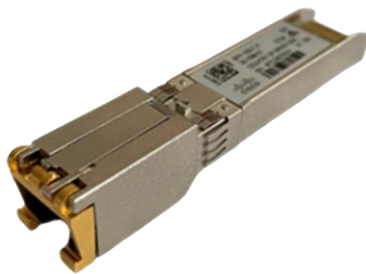
Figure 2. Cisco SFP+ 10GBASE-T module with RJ-45 connector
